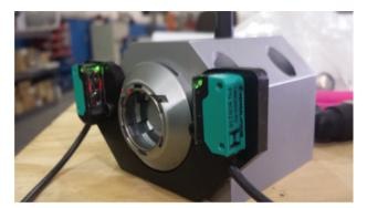
**Machine Components**Example of in-process inspection integrated into tooling.
