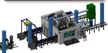
Example of automated turning & drilling system
